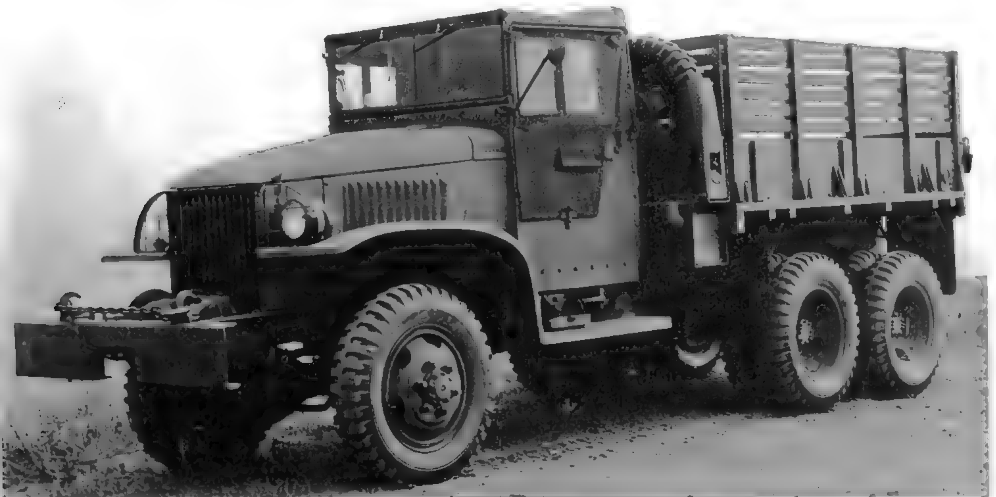
A driver's-side view of the open-cab CCKW-352. The liquid container bracket on the driver's side running board was also a late-war addition to the production line. (Photo courtesy of Bryce Sunderlin collection)
